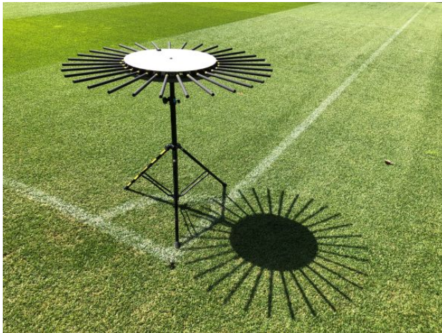
The prototype AMBEO Sports Microphone Array for 360° sound will be on display.
